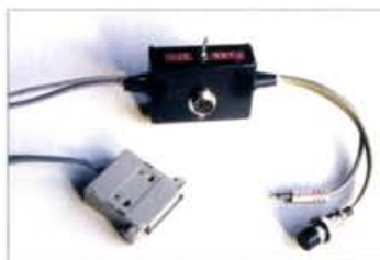
Fig. 2: (a) Denis G3KCR's change-over box circuit which he built himself. (b) Denis' change-over box circuit in diagrammatical form.
