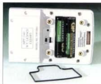
Fig. 2: Removing the back and its sealing gasket, reveals switches for the transmit channel and measurement scale, along with the small helical-wound 418MHz antenna, visible in the 'window'.
