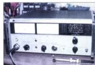
Fig. 7: The Hewlett-Packard HP4084 vector impedance meter is a stand-alone instrument and does not require any additional equipment to make the measurement.
