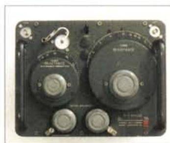
Fig. 4: A commercial r.f. impedance bridge, from the General Radio Company. This instrument needs a signal source, such as a signal generator and a receiver to detect when the bridge is balanced.
