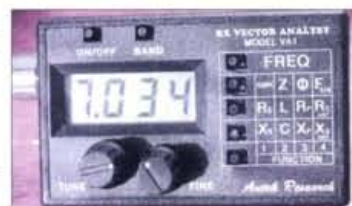
Fig. 6: The Autek RX Vector Analyst VA1, a tiny instrument that can measure a wide range of r.f. parameters
